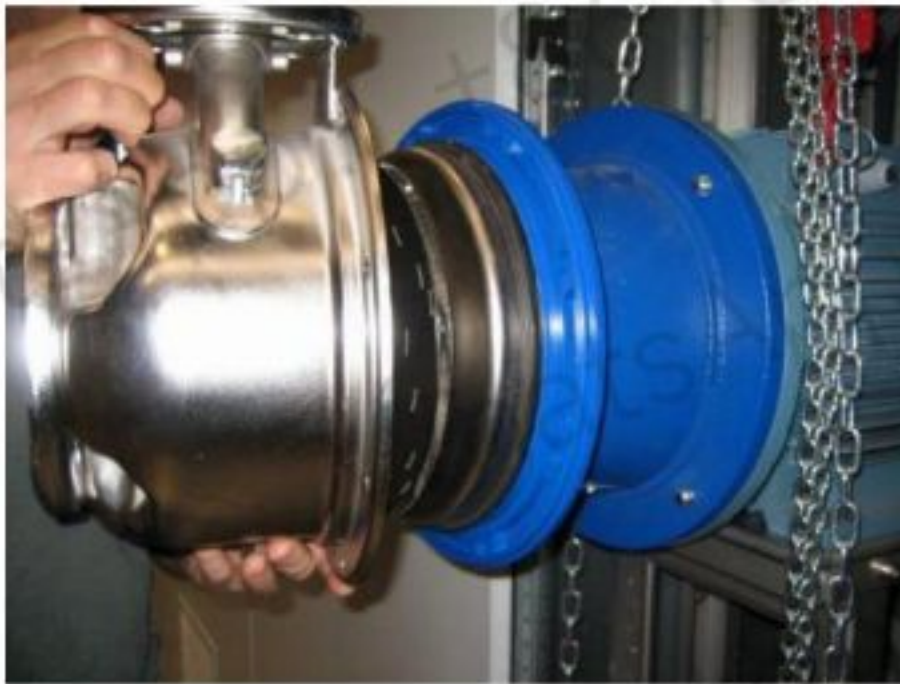
Figure 10–82 Opening pump case
